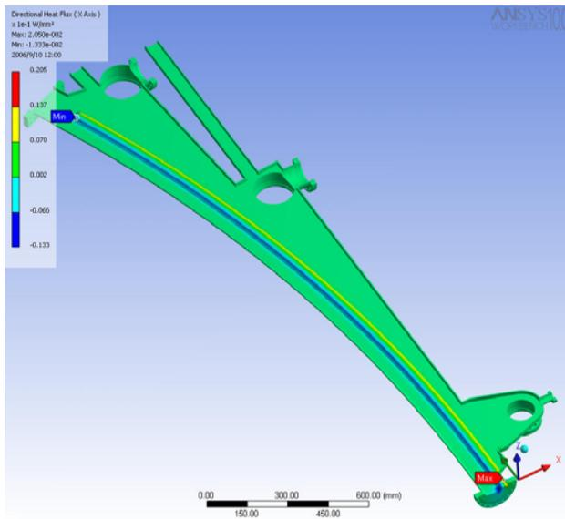
**Thermal Load Due to Radiation Heat**
