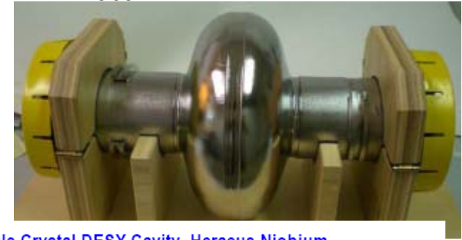
Single Crystal DESY Cavity, Heraeus Niobium 112 micron bcp 1:1:2
