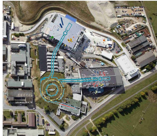
Figure 2: Aerial view of ISIS showing the new extracted proton beamline and the building for Target Station 2.
