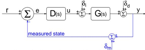
Figure 2: First order closed loop block diagram
