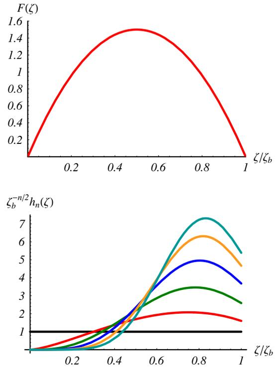
Fig. 1: Parabolic charge distribution from Eq. (13) with  $\alpha = -6$  and functions  $h_0(\zeta)$  to  $h_6(\zeta)$ .
