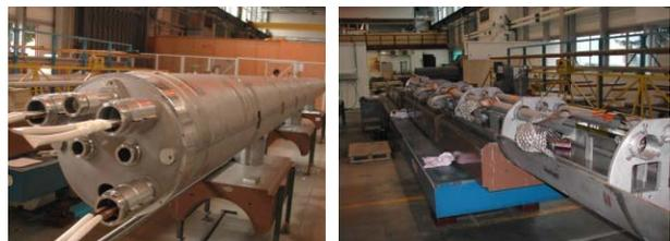
Figure 1: Cold Mass inside the Connection Cryostat.
