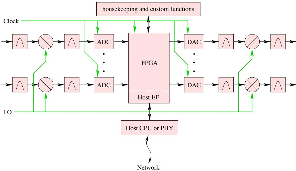
Figure 3: Familiar block diagram, including RF signal conditioning.
