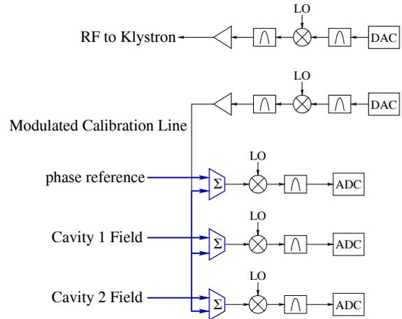
Figure 4: Insertion of phase calibration signal.
