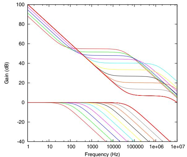
Figure 2: Frequency domain strategy for closing feedback loop.
