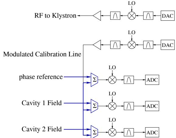
Figure 4: Insertion of phase calibration signal.
