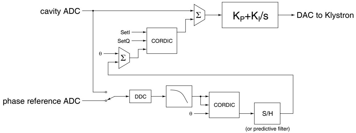
Figure 5: Digital signal processing of cavity and reference signals.
