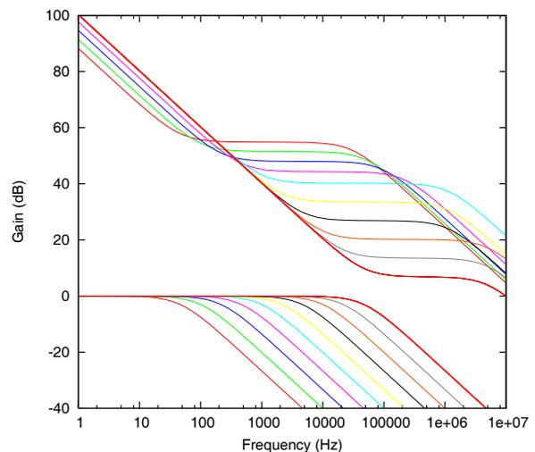
Figure 2: Frequency domain strategy for closing feedback loop.
