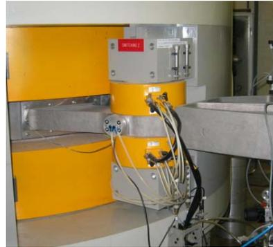
Figure 7: Cyclone30 switching magnet.
