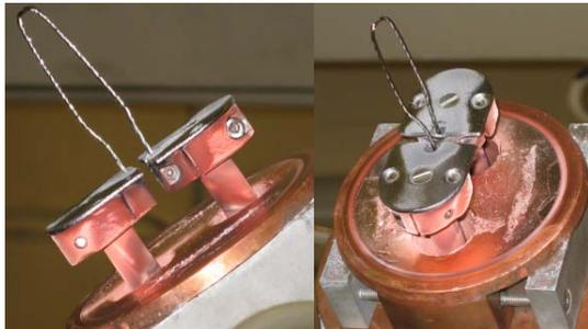
Figure 3: LHS shows hairpin tungsten filament and exposed support posts. RHS shows backplate with two cusp magnet rows used in the Cyclone30.
