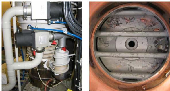
Figure 2: LHS shows Cyclone30 ISIS diffusion pump. RHS shows ion source with hydro-carbon debris.
