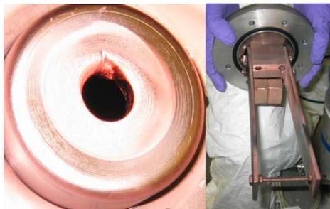
Figure 4: LHS shows wear in source ground lens. RHS shows permanent steering magnet in Cyclone30.
