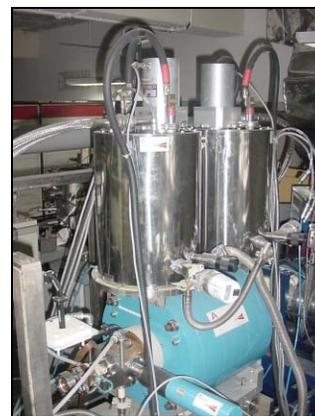
Figure 1. View of the High Temperature Superconducting ECR Ion Source, PKDELIS
