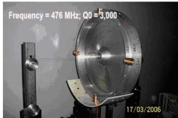
Fig 2 Aluminium prototype of pre-buncher cavity
