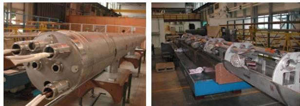
Figure 1: Cold Mass inside the Connection Cryostat.
