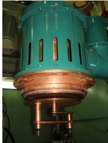
Figure 2: RF generator with power input loop
