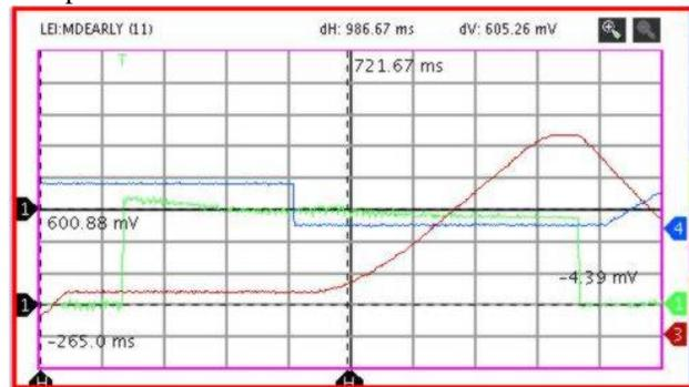
Figure 1: The "early ion beam" in LEIR (200ms/div). The red trace is the main bending field, the green trace is the beam current ( $8 \cdot 10^7$  ions/div), the blue trace is the electron cooling cathode voltage which is reduced just before the ramp.
