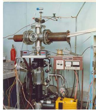
Figure 2. Photograph of the experimental setup of Low Pressure Sparkgap
