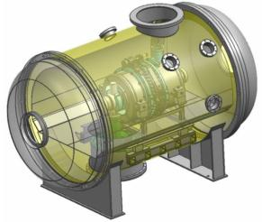
Figure 5: Conceptual layout of the single cavity module for the testing of the high energy components.
