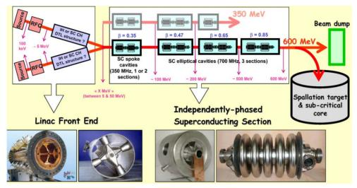
Figure 2: The reference accelerator scheme for the ETD/XT-ADS.
