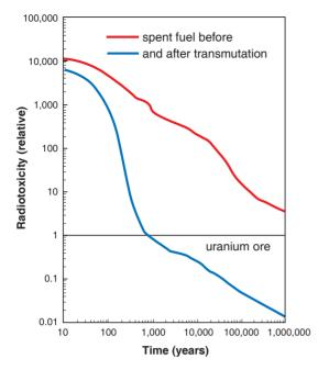
Figure 1: Ingestion radiotoxicity of spent nuclear fuel, before and after partitioning and transmutation, compared to the uranium ore level. From Ref. [1].
