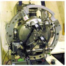
Figure 4: The spoke cavity equipped with the cold frequency tuner in the support frame of the cryostat.
