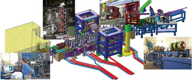
Figure 3: Scheme of the IPHI injector, and pictures of the components during their installation at Saclay.
