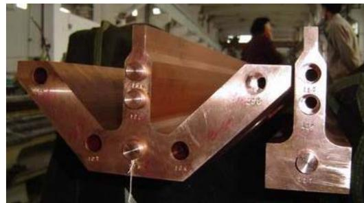
Figure 5: The water cooling channels of 1.2m long were drilled through the pieces and plugs were used to cover them on each end by brazing.
