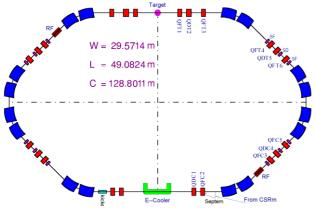
Figure 1: The layout of the CSRe
