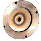
Figure 1: the photograph of beam baffle
