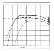
Figure : 4 See from top, traces of Klystron beam voltage at 110kV @10kV/div., klysron beam current and output microwave pulse power 2.6 MW delivered to microtron cavity
