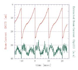
Figure 5: Time distribution of extracted beam for 100 pps operation. A ring current is also shown (upper line).
