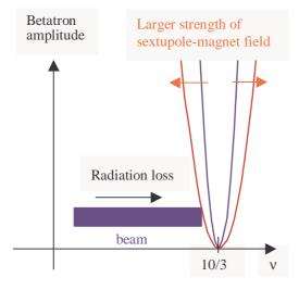
Figure 2: Schematic diagram of beam extraction.
