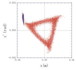
Figure 3: Horizontal phase space distribution at a wire septum. The extracted beam (x<-0.03m) is also shown.
