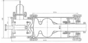
Fig. 2 Configuration of DC-SC photocathode injector
