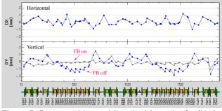
Figure 7: Beam positions with and without the feedback, which were taken 24 hours after the last COD correction.
