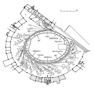
Figure 2: Layout of the Photon Factory storage ring.
