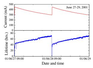
Figure 6: Beam current and beam lifetime during two days.
