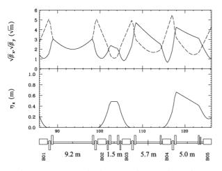
Figure 9: Beam optics in the straight sections after the upgrade.
