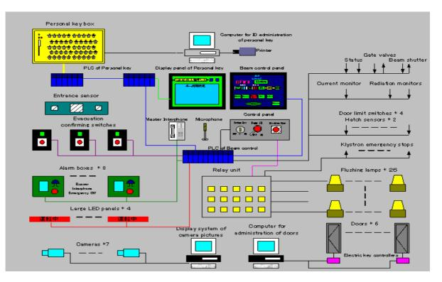
Fig.2 Control of the beam switch and construction of the safety system
