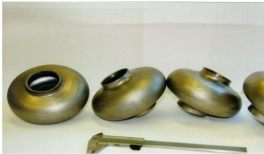
Fig.9 Single cell cavities in reduced size (60% of TESLA shape) produced by hydroforming without intermediate annealing and intermediate constraint
