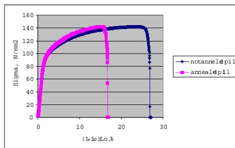
Fig. 8. Strain-stress behavior of samples from the tube with annealed and not annealed pills.
