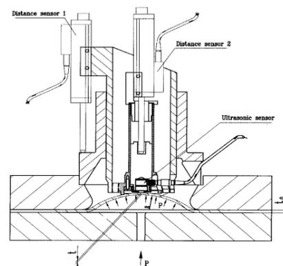
Fig. 1. Scheme of the bulging device
