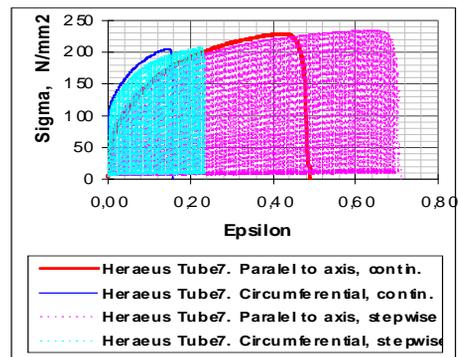
Fig.6 Comparison of the traction test in continuous and pulse regime
