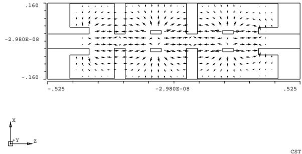
Figure 2: Electric Field in Spoke Cross Bar Cavity
