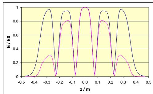
Figure 7: Electric Field Distribution in Spoke 5-Cell Ladder Cavity Depending on End Region Tune
