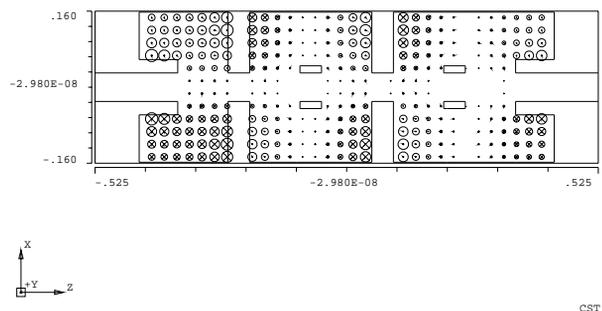
Figure 3: Magnetic Field in Spoke Cross Bar Cavity
