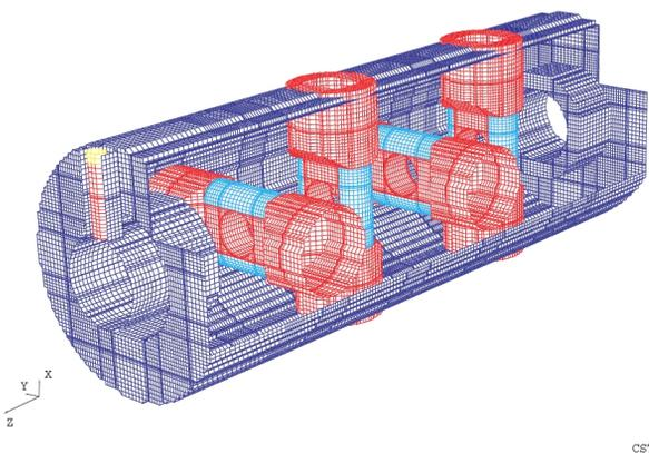
Figure 1: Spoke Cross Bar Cavity Geometry
