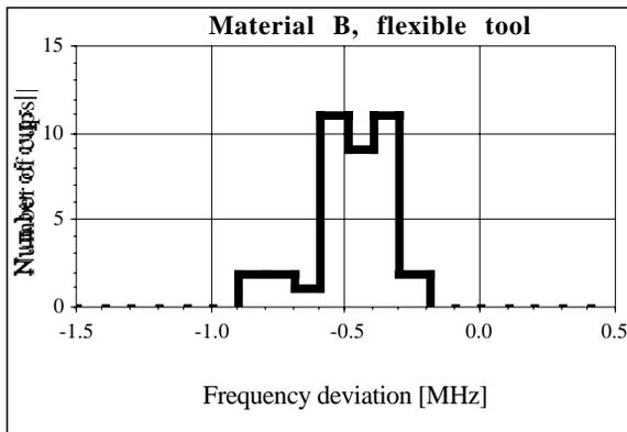
Figure 6: The frequency statistics of cups fabricated by pressing the sheet with a resilient cushion over an inner metal tool.
