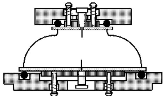
Figure 4: Photo and schematic cross-section drawing of the test device for the frequency measurements of dumb-bells (left) and cups (right)
