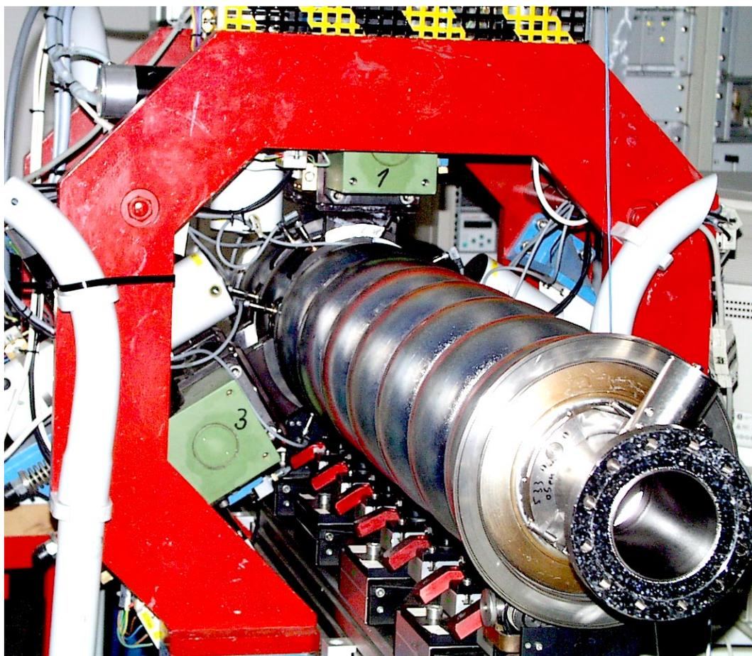
Figure 2: Photo of the computerized tuning machine
