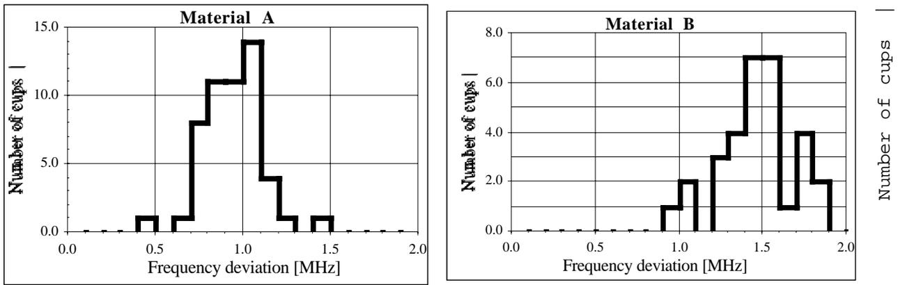
Figure 5: The frequency statistics of 90 (left) and 29 (right) cups from two different materials. Deep-drawing was done with an inner and outer metal tool.
