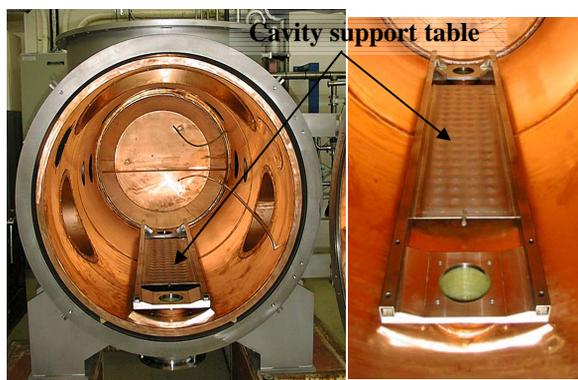
The support table is cooled at 4.2 K with liquid Helium, and is isolated from the vacuum tank at 300 K by epoxy-glass posts heat sunk at 80 K by the thermal shield.
