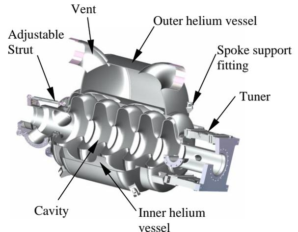
Figure 1: Cut-away of cavity installed in helium vessel
