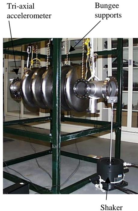
Figure 5: Test Setup for Stage 1
