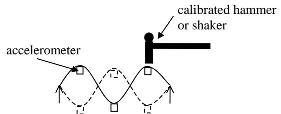
Figure 3b: Multiple measurement points necessary to capture mode shapes
