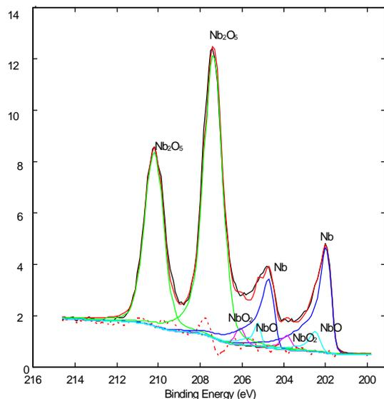
Figure 1 Deconvolution of the Nb3d line for one of the samples exposed to air; to reproduce the line-shape four chemical states (Nb, NbO, NbO<sub>2</sub>, Nb<sub>2</sub>O<sub>5</sub>) are necessary.
