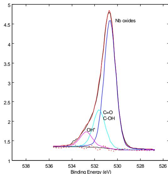
Figure 2 Deconvolution of the O1s line for one of the samples exposed to air; the spectrum is reproduced by three chemical states (Nb oxides, C=O and C-OH, OH<sup>+</sup>).
