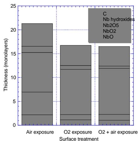
Figure 5 In-depth chemical composition of the samples exposed to air and to dry O<sub>2</sub> (up to saturation). The last bar represents the in-depth composition of the dry oxidised samples exposed for a long time (about 10 days) to air after the dry O<sub>2</sub> exposure. The errors on the thickness values are between  $\pm 0.1$  and  $\pm 0.3$  monolayers.
