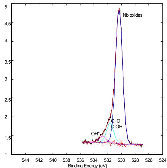
Figure 3 Deconvolution of the O1s line for one of the samples dry oxidised; the spectrum is reproduced by three chemical states as in Figure 2, but the contribution of the OH<sup>+</sup> signal is strongly reduced.
