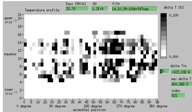
Figure 4: Temperature map at  $E_{acc} = 33$  MV/m before in-situ bakeout.
