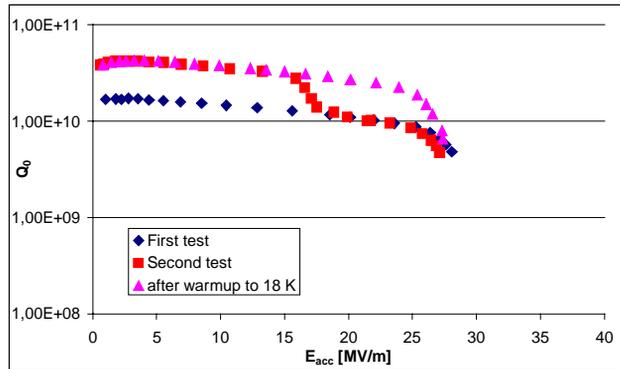
Figure 2: Q-degradation during multipacting. The first breakdown events are typically seen at 17 MV/m.
