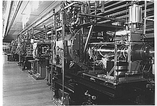
Figure 10: Four SC damped cavities installed in HER.
