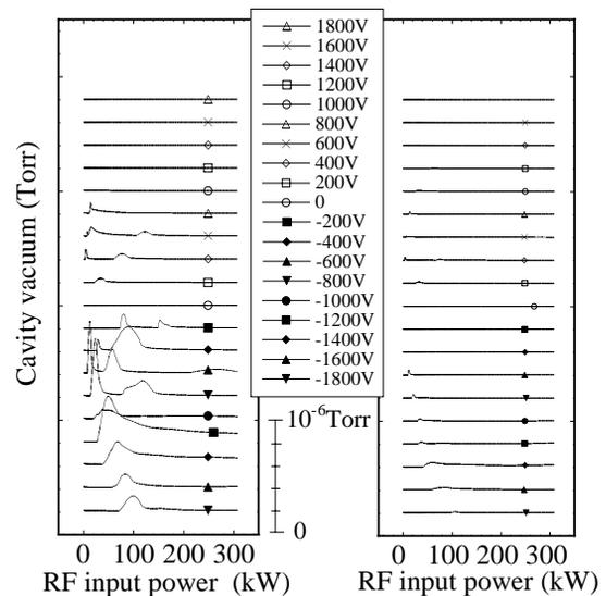
Figure 8: Mapping of vacuum pressure versus input power, scanning the power for the various bias voltages up to  $\pm 1.8$ kV.
