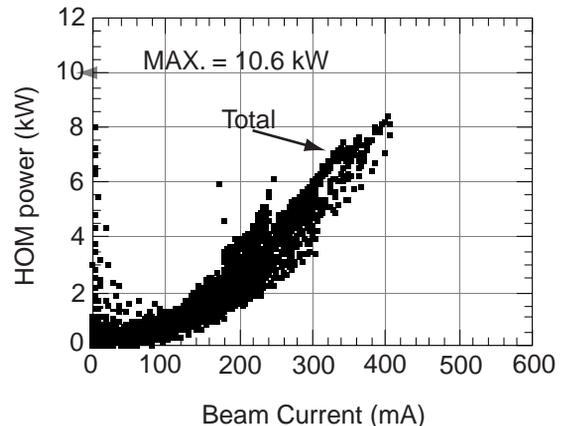
Figure 7: The HOM power absorbed by the dampers.
