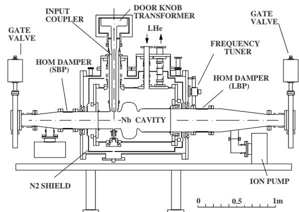
Figure 2: A sectional view of the SC damped cavity.
