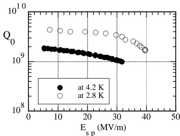
Figure 9: Q-E of the full size model cavity.
