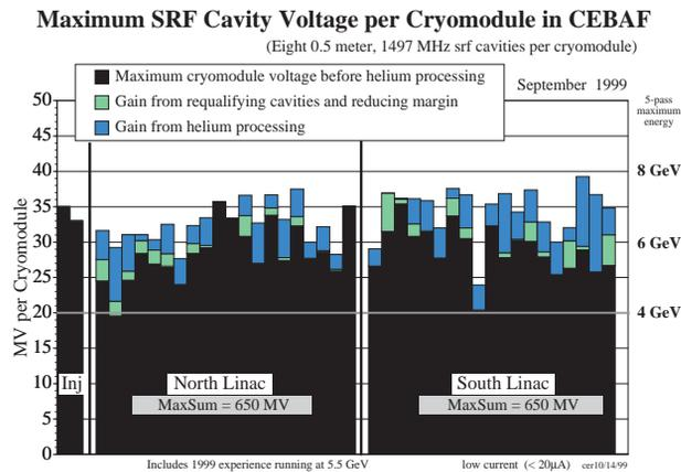
Figure 3. Peak capability of the CEBAF cryomodules.
