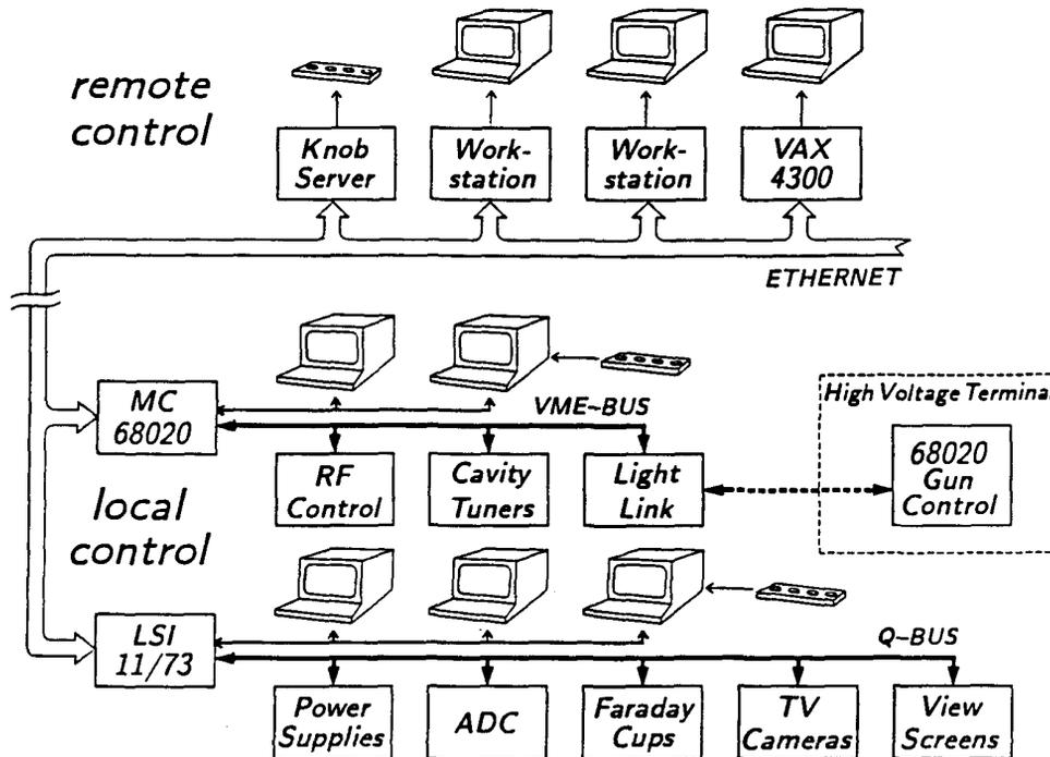
Fig. 2 Accelerator Control System
