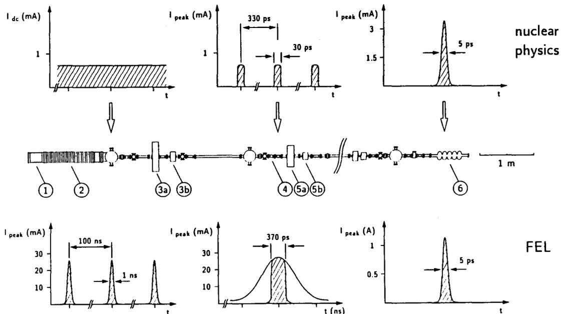
Fig. 5 Time structure of the beam for 3 GHz cw (nuclear physics) and 10 MHz cw (FEL) mode of operation in the injection beamline. The figures denote: (1) electron gun, (2) 250 kV preacceleration, (3a) 600 MHz-, (3b) 3 GHz-chopper cavity, (4) chopper aperture, (5a) 600 MHz-, (5b) 3 GHz pre-buncher cavity, and (6) 5-cell capture section.
