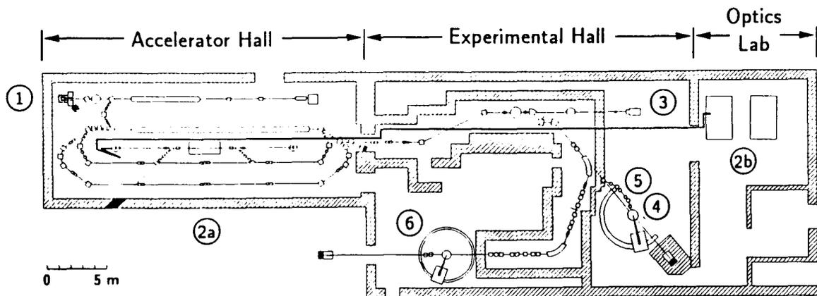
Fig. 1 *Layout of the S-DALINAC and its experimental facilities: (1) low energy channeling, (2a) FEL with (2b) optics lab, (3) high energy channeling, (4) QCLAM spectrometer, (5) bypass for  $180^\circ$  scattering, (6) energy loss spectrometer.*
