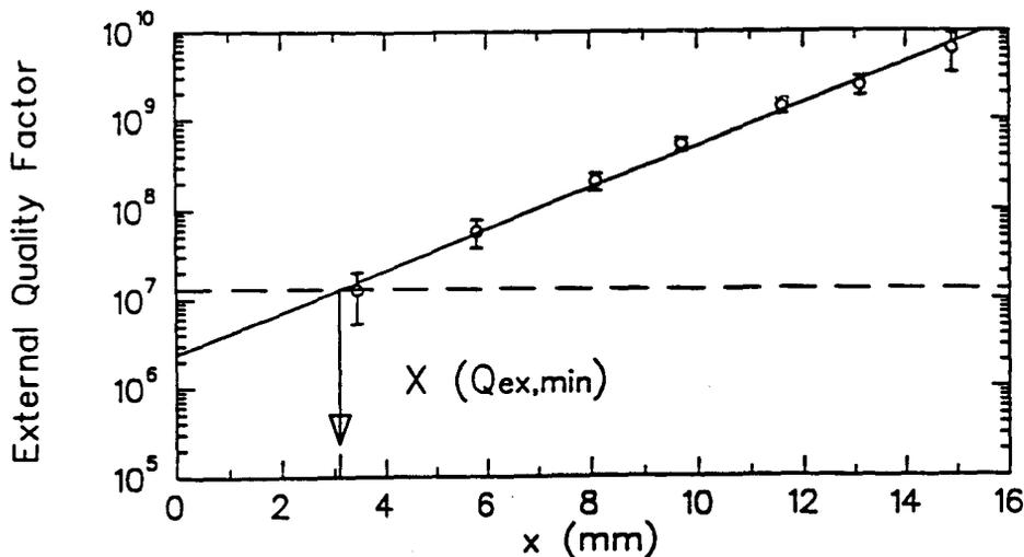
Fig. 4 Performance of the variable input coupler at 2K;  $x$  denotes the spacing between the center conductors of RF input line and intermediate coaxial resonator.
