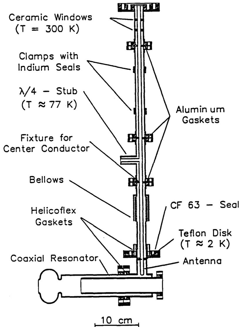
Fig. 3 Variable input coupler with 7/8" coaxial RF input line
