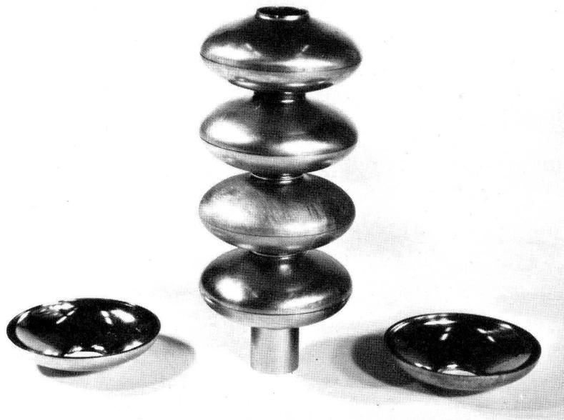
Fig.6 Superconducting RF-structure made of Nb sheet prior to welding.
