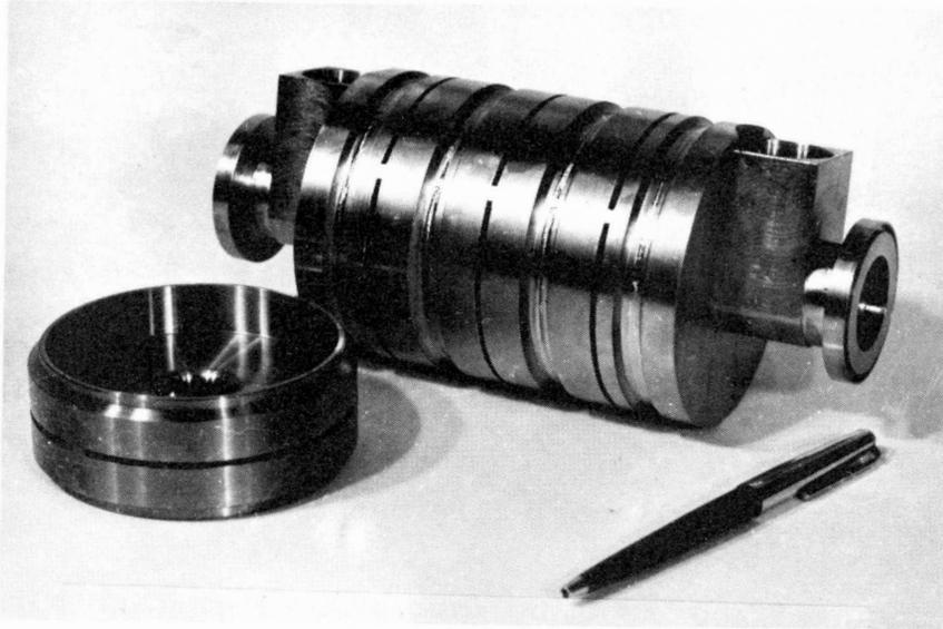
Fig.2 Capture section made from casted Nb.
