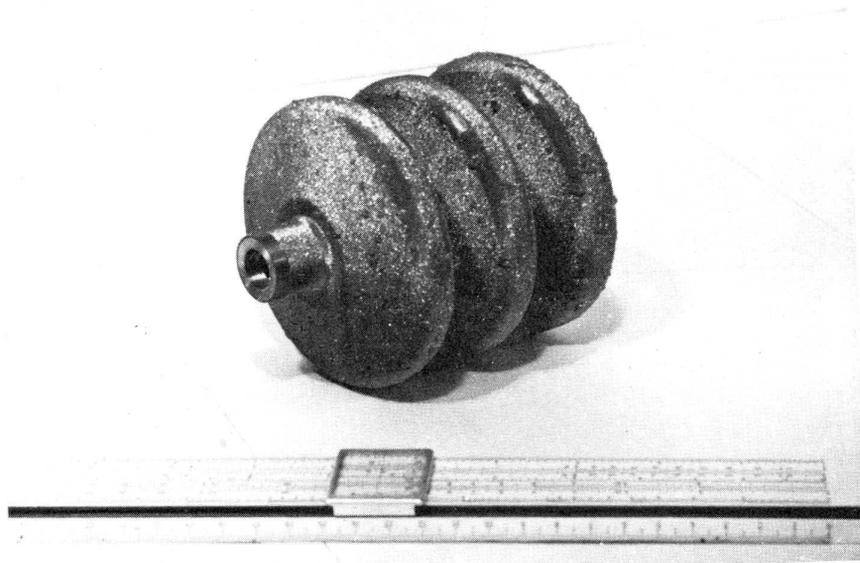
Fig.1 Prototype of a capture section produced by galvanoplastic method.
