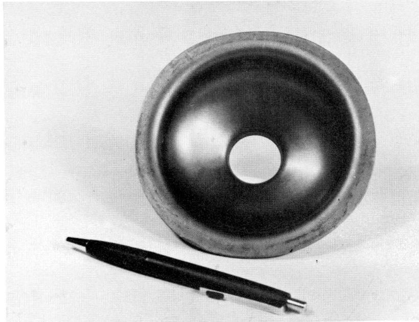
Fig.4 Half-cell of the RF-structure after deep-drawing.
