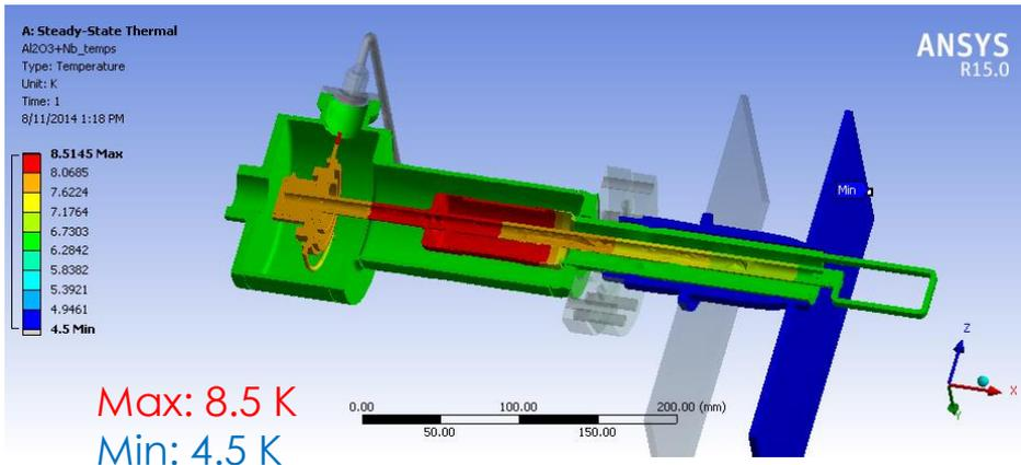
The braze material at the sapphire – Nb cuff joint is InCuSil, which is normal conducting at 4.5 K.
