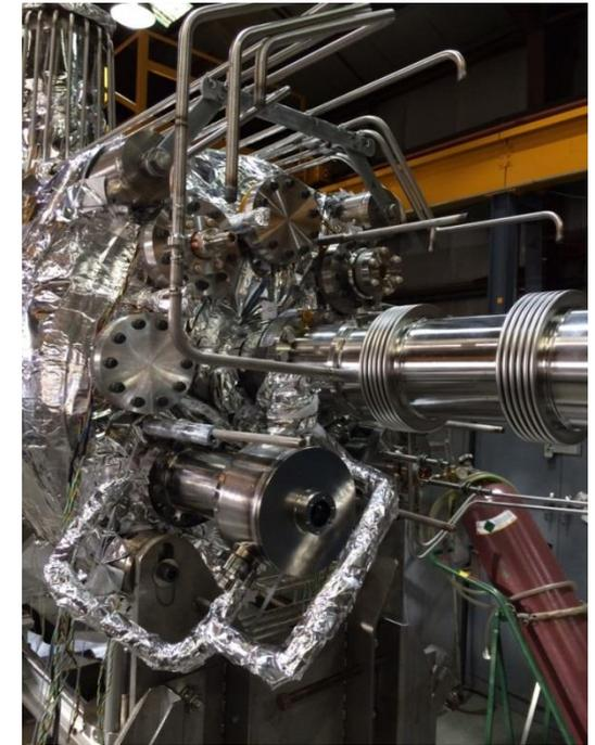
The HOM coupler has a sapphire RF window that is designed for separating the high-pass filter section from the cavity vacuum.
