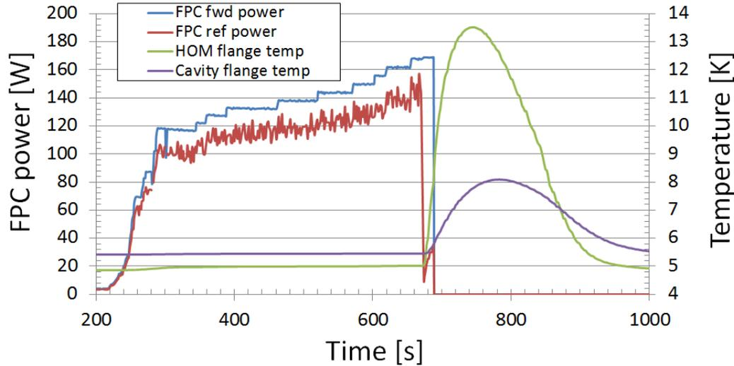
The cavity voltage was limited by a quench in the HOM coupler assembly. The maximum reached cavity voltage was:
