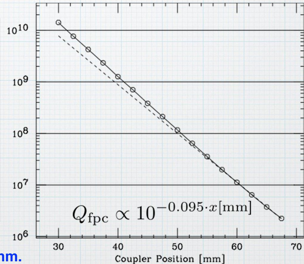
**Antenna stroke should have  $\pm 5$  mm.**
