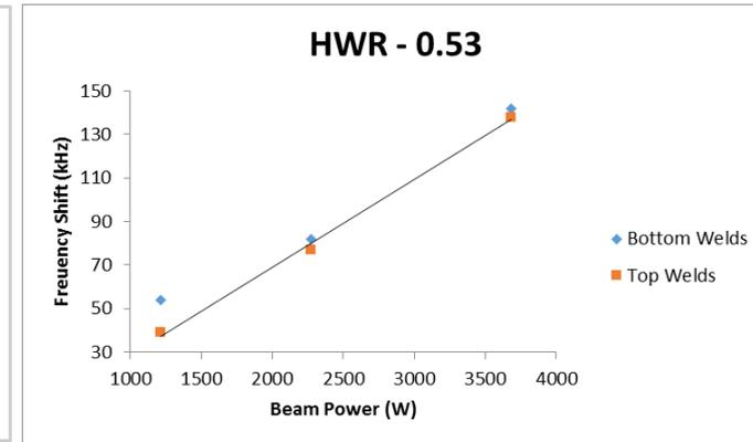
Electron-beam power calibrations for virtual welding of half-wave cavities ( $\beta_0 = 0.29$  and  $0.53$ ) prior to helium vessel integration
