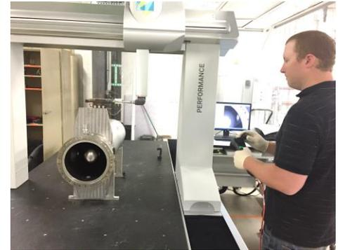
Dimensional inspection using Coordinate Measuring Machine (CMM)
