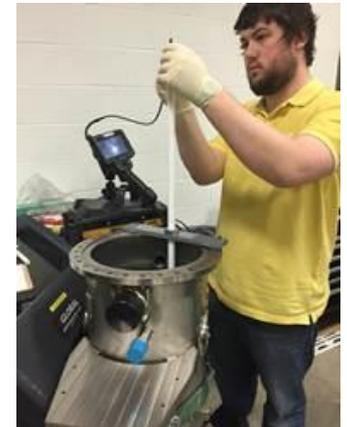
Internal boroscope inspection
