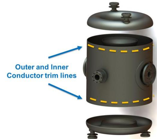
HWR frequency tuning using OC and IC stack and trimming
