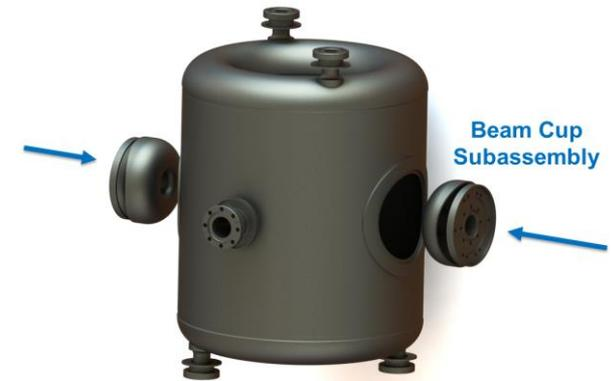
HWR frequency tuning using beam cup positioning
