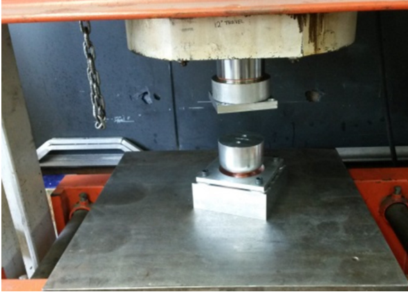
Forming press is used for making halves of each cell
