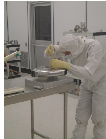
PBG rods are made separately and then fitted in the cell
