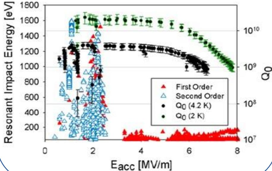
Multipacting activity predicted below 2.5 MV/m using Track3P. First test verified this. Easily processed.
