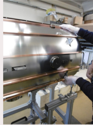
Magnetic shield (2-layer Cryophy, actively cooled)
