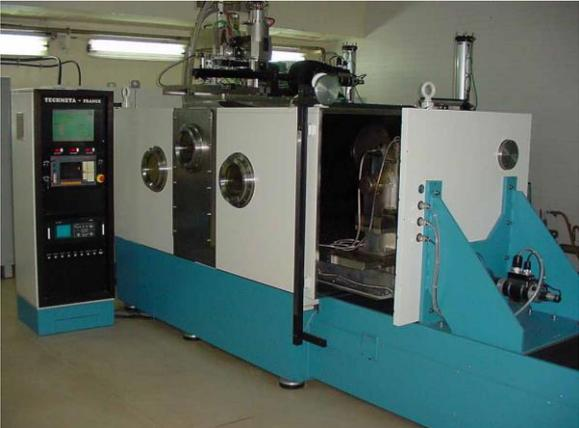
Electron Beam Welding facility
