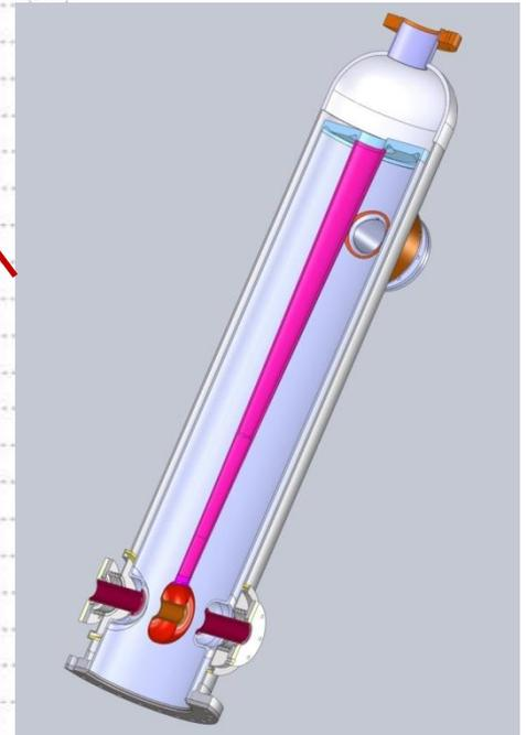
The new niobium Low Beta Resonator (LBR) developed for the LBM.
