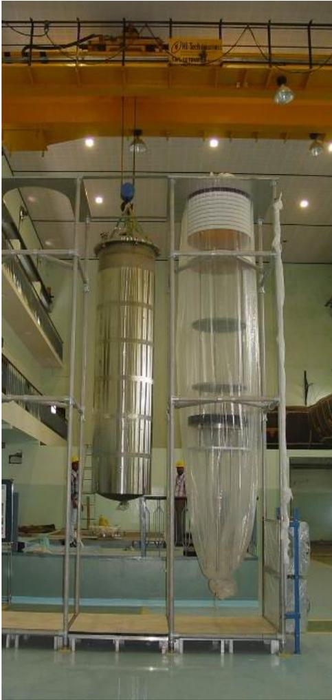
Cryostat & Cavity Insert Assembly
