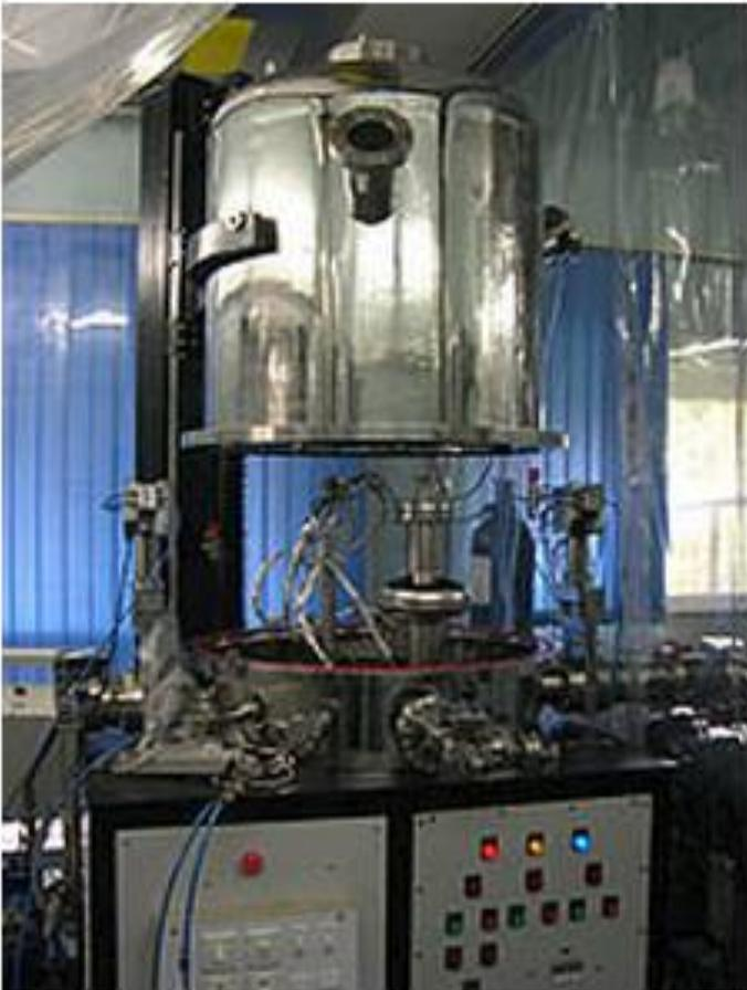
A novel technique of fabrication of SCRF cavities using Nd-YAG laser welding process, has been developed at RRCAT. The process has received patent from Japan.
