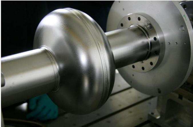
1.3 GHz TESLA-type cavity no. 3
