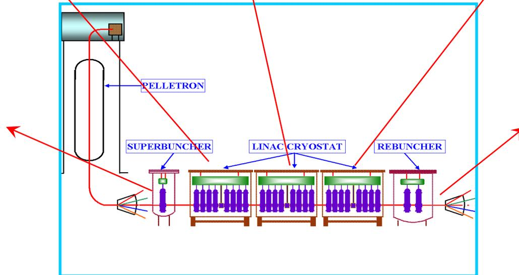
Consists of 27 identical Quarter Wave resonators,  $\beta_0 = 0.08$ ,  $f_0 = 97$  MHz
