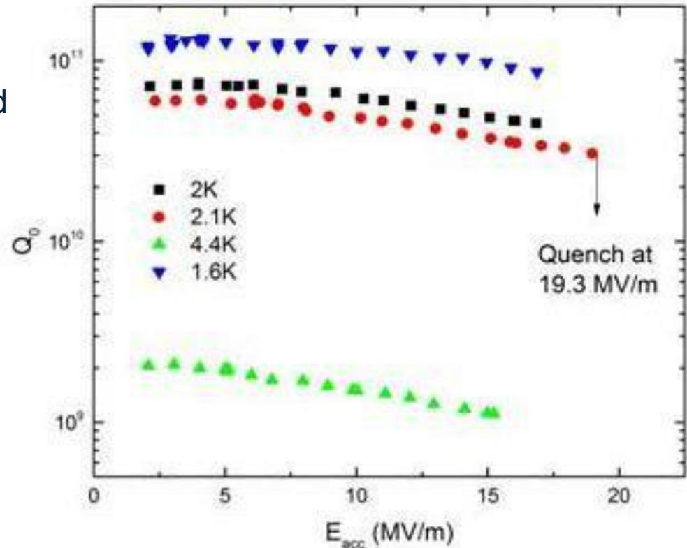
Performance of the 650 MHz,  $\beta=0.9$  Single Cell Niobium Cavity tested at Fermilab. The cavity achieved 19.3 MV/m gradient at  $Q_0=3 \times 10^{10}$ , exceeding the design goal of 17 MV/m at  $Q_0 > 2 \times 10^{10}$ .
