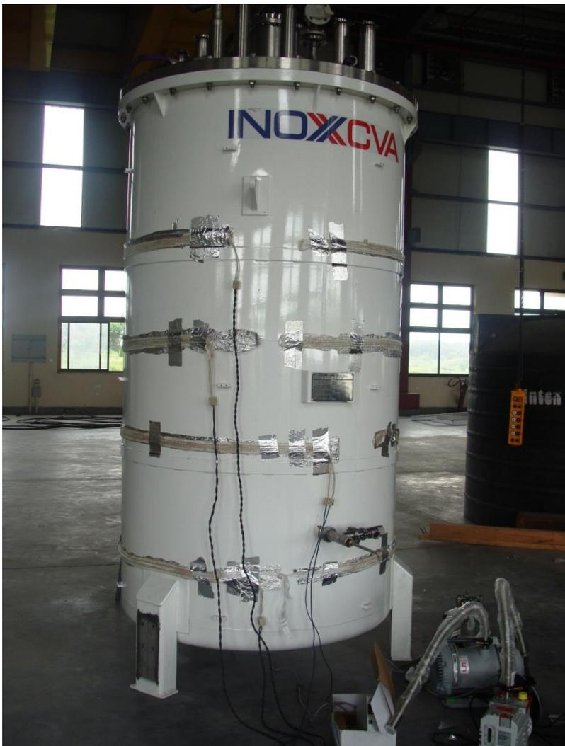
• VERTICAL TEST CRYOSTAT (FOR 650 MHz,  $\beta=0.61$ , 5-CELL SRF CAVITY) HAS BEEN DESIGNED IN-HOUSE AT VECC AND GOT FABRICATED BY INOX-INDIA AND INSTALLED AT VECC (RAJARHAT CAMPUS).
