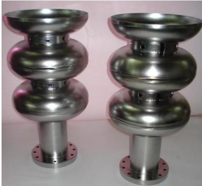
Two halves of the 5-Cell Cavity.
