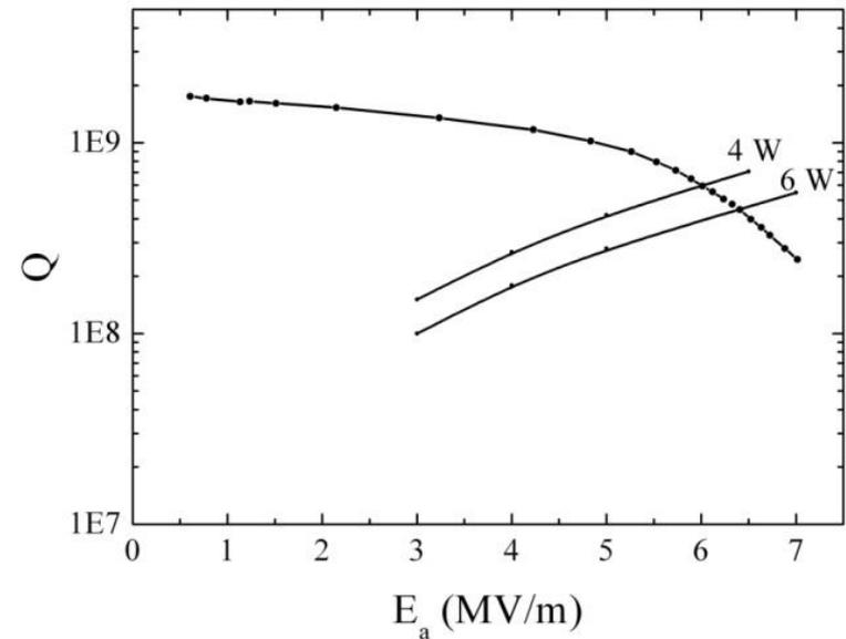
Typical performance of an inductively built QWR at 4.2 K.
