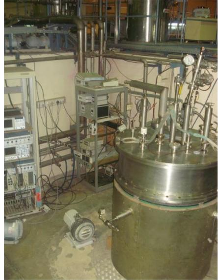
Test Cryostat (partially buried)
