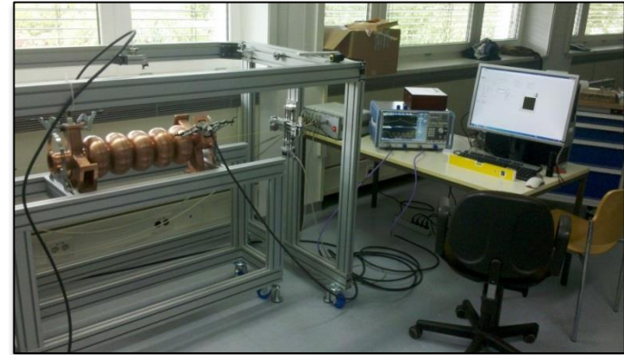
Copper prototype (1.5GHz) (5 WG+1 FPC) with Rotary mechanical flanges
