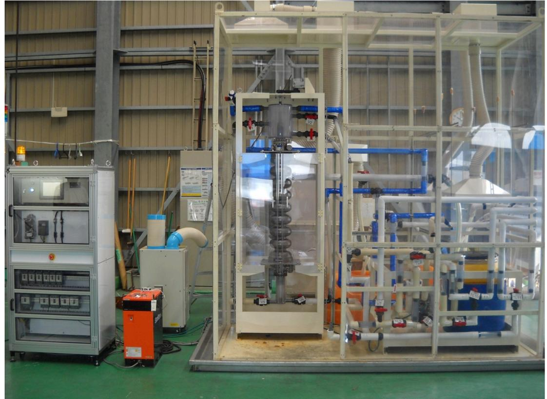
✧ Both setups were prepared with PVC materials in order to reduce cost of surface treatment of cavities in mass production.
