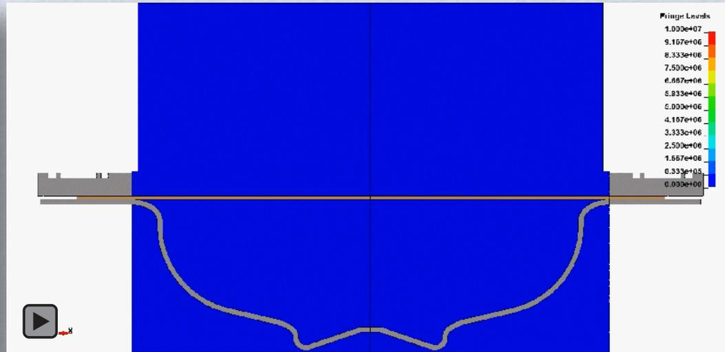
Simulations is used to define the number and position of discharges and to select the energy level.
