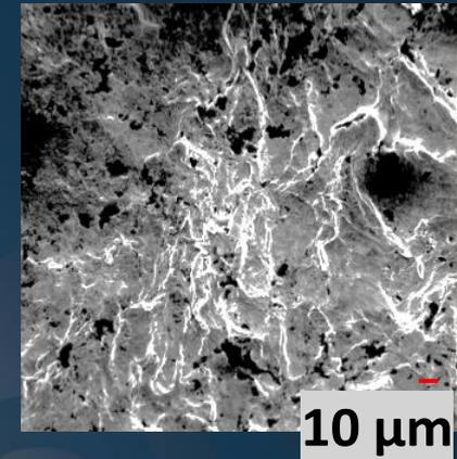
Pb-layer after the 2<sup>nd</sup> laser cleaning
