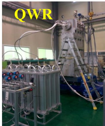
P&ID and photo for QWR cryomodule test apparatus
