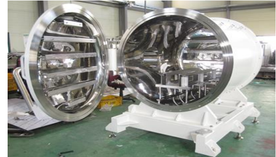
Vacuum Furnace (completed)
