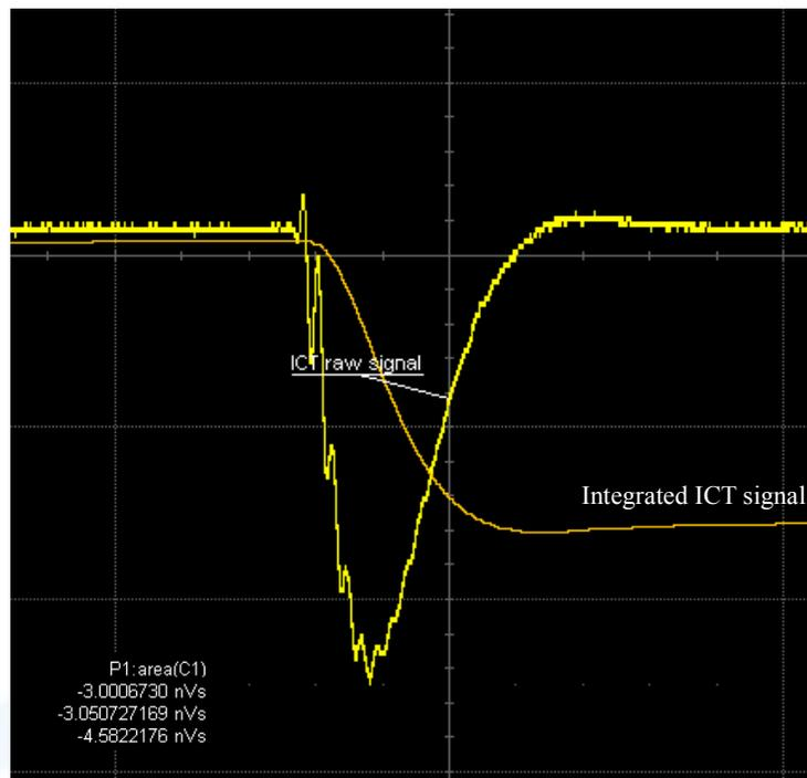
Oscilloscope trace of a raw signal from ICT and its integral. The integrated signal corresponds to bunch charge of 2.4 nC.
