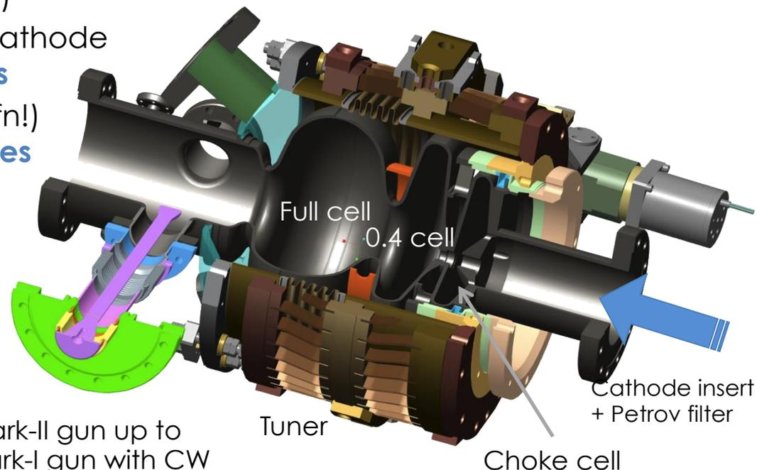
Twin CW RF couplers (Mark-II gun up to 115 kW. Shown here: Mark-I gun with CW modified TTF-III couplers for 10 kW CW)
