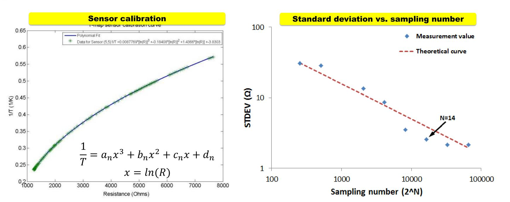
Increasing measurement sampling number (2<sup>N</sup>) is an effective way to reduce noise from the electronic system. The standard deviation is reduced to about 2Ω, when N is set to 14, corresponding to a sampling number of about 16000. The noise from the electronic system is about 200µK in 2K helium bath; and 67µK in 1.6K helium. The total scan time is about 100s and the total noise of the T-map system is about 1mK. Multi-cell T-map has achieved the initial target resolution.
