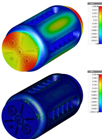
Figure 5: Maximum deformation (top) and von Mises stress (bottom) of the cavity due to the evacuation process.
