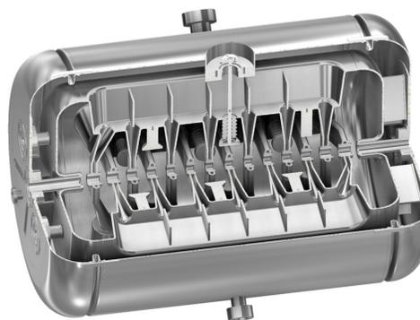
Figure 1: Layout of the sc 217 MHz CH cavity.
