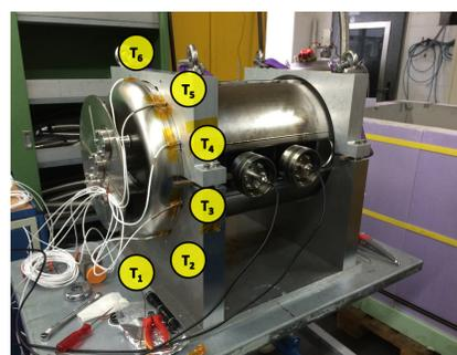
Figure 3: Setup with six temperature sensors to measure the frequency shift during cool-down with LN<sub>2</sub>.
