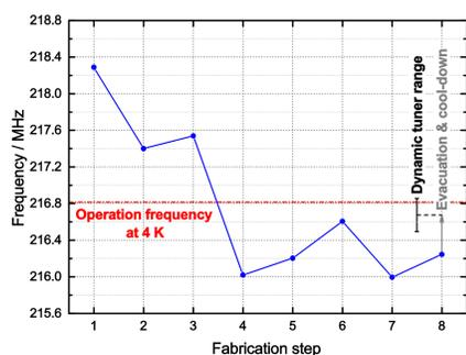
Figure 2: Measured frequency of the cavity during each fabrication step.
