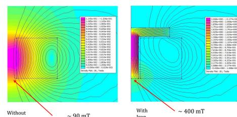
Fig 4: Field lines before and after the insertion of iron core inside the coil to enhance the magnetic field  $>150$  mT on the sample.
