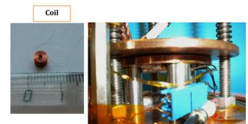
Fig 2: a) Coil ( $r=0.2$ cm); b) sample holder
