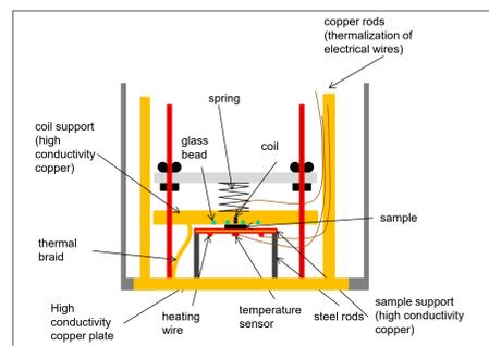
Fig 1: Schematic of Local Magnetometer
