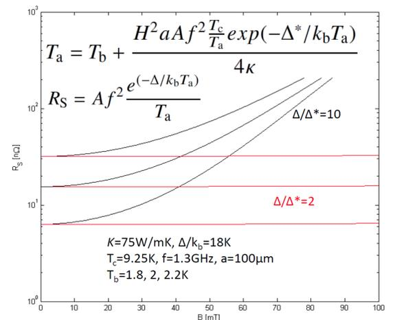
Figure 4: Surface resistance of the area around a defect with suppressed gap value as a function of applied magnetic field. The model is inspired by the model for thermal breakdown from Padamsee et al. [RF superconductivity for accelerators. Wiley, Weinheim, 2. edition, 2008] (see Fig.5). It assumes a defect with lowered gap value of radius  $a$ . From the heat flow the surface resistance from the area around the defect is calculated by solving the equations displayed above numerically.
