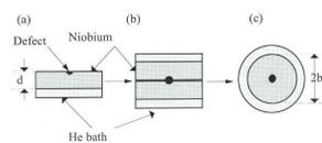
Figure 5: The geometry of our model is inspired by Padamsee et al. We use the idea of modeling a hemispherical defect by heat source inside a sphere.
