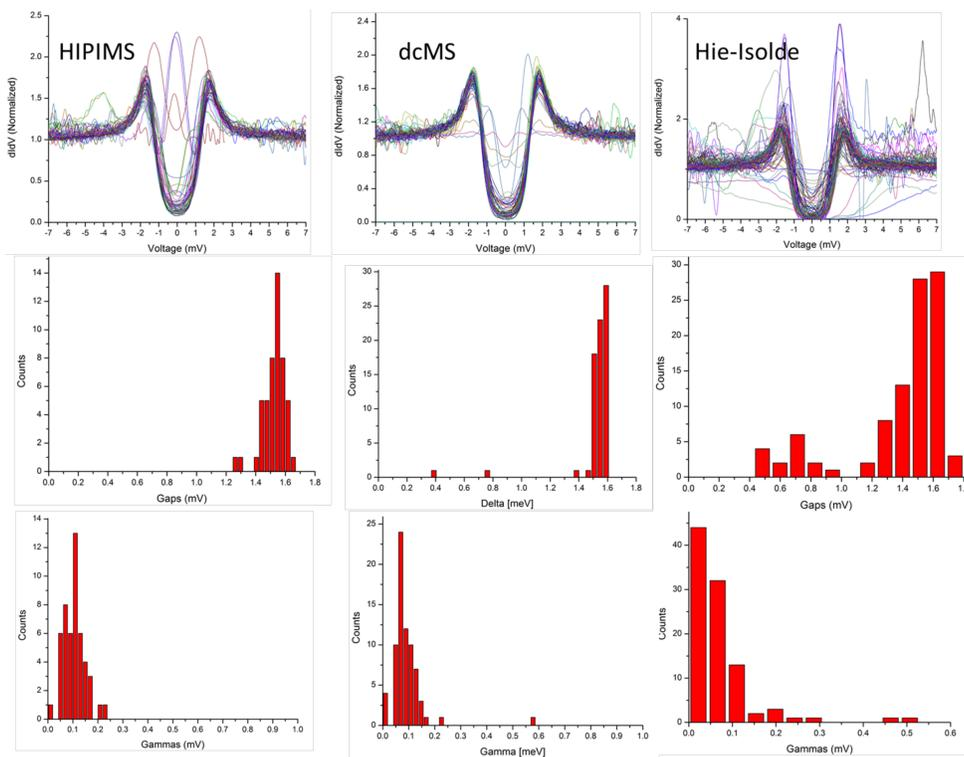
Figure 3: Tunneling spectra of about 80 junctions each for three Nb/Cu samples (top). Corresponding gap values (middle) and phenomenological quasiparticle lifetime broadening parameter (bottom) extracted from fits to the Blonder-Tinkham-Klapwijk (BTK) model [C. Dynes et al. Phys. Rev. Lett., 41:1509, 1978, G. E. Blonder, Phys. Rev. B, 25:4515, 1982]
