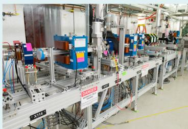
The 50 MeV beam transport line immediately follows CC2. The electron beam passes through a quadrupole doublet for controlling the beam size for emittance measurements, a matching section, and then into a 4-dipole chicane for bunch compression ( $R_{56} = -0.18$  m), and a matching section, thence into a 22.5° vertically downward bending dipole. This dipole, upstream of the absorber, serves as the low energy spectrometer. The 50 MeV beam absorber is capable of accepting up to 550 W of beam power.
