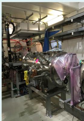
**Capture Cavity 1 (CC1)** upgrade work is now completed. The cryomodule has been installed on the FAST beam line. CC1 re-commissioning and operation is expected to occur in late 2015/early 2016. Based on cavity horizontal tests it is expected to operate at gradients up to 29 MV/m.
