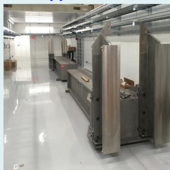
To minimize stray magnetic fields, the cryomodule support girders and hardware within them are fabricated from 316L stainless steel. Each girder bears half of the cryomodule weight, 8,130 lbf.
