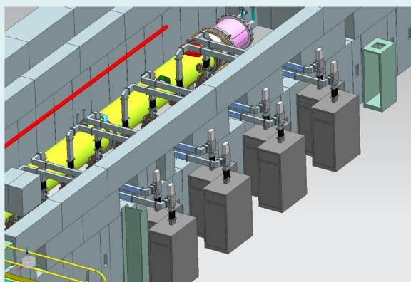
Each cavity will have its own RF source. Solid state amplifiers (SSA's) will be located outside and immediately adjacent to the test cave. Circulators to minimize reflected power back to amplifiers are mounted above each SSA. Individual waveguide runs will enter the cave near the cave ceiling height and then drop vertically above the respective coupler port. The vertical sections are designed for rapid removal to allow sufficient clearance to crane cryomodules in and out between tests.
