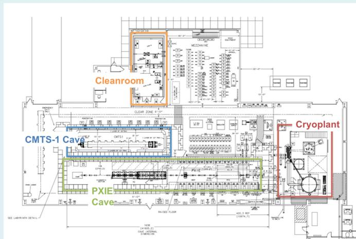
CMTF consists of two new adjoined buildings located adjacent to the existing NML building, and together with NML comprises a world-class facility for testing SRF components with and without beam.
