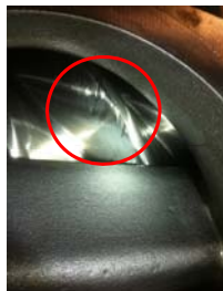
Left to right: Damage to compressor airend lobes, Normal oil colour (left) versus damaged airend oil colour (right), and damaged MCTL cold GHe return pipe bellows.
