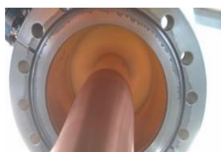
The vacuum side of the cracked ceramic turns on a uniform yellow color.
